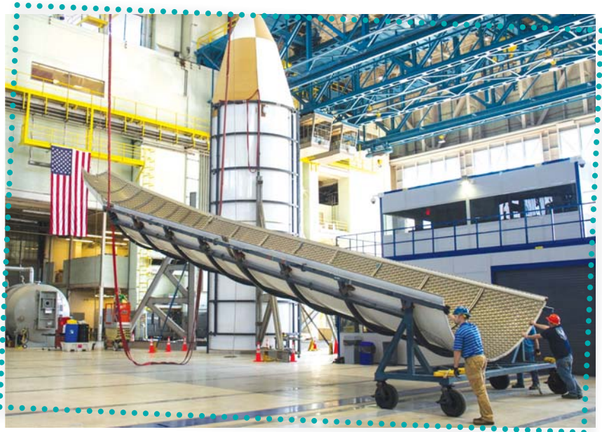
Air Force Research Laboratory engineers and technicians from the Structural Validation Branch of the Aerospace Vehicles Division, Aerospace Systems Directorate, partnered with museum restoration crews to assemble a 60 foot tall payload fairing from the Titan IVB space launch vehicle Feb. 29-March 2, 2016. (U.S. Air Force photo by Ken LaRock)
