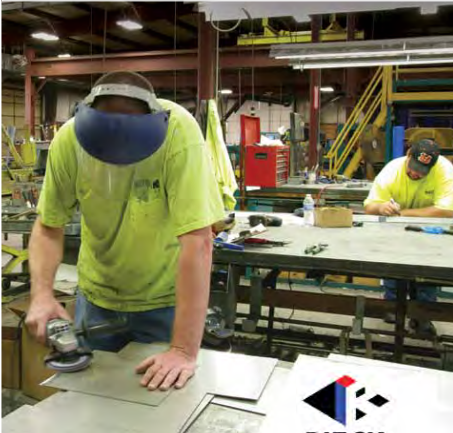
Rieck sheetmetal workers grinding stainless steel.
